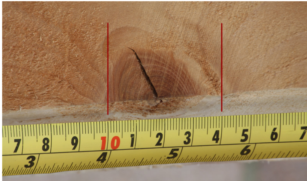
Figure 3: [SOP_SHO 004] Maximum size of knots
