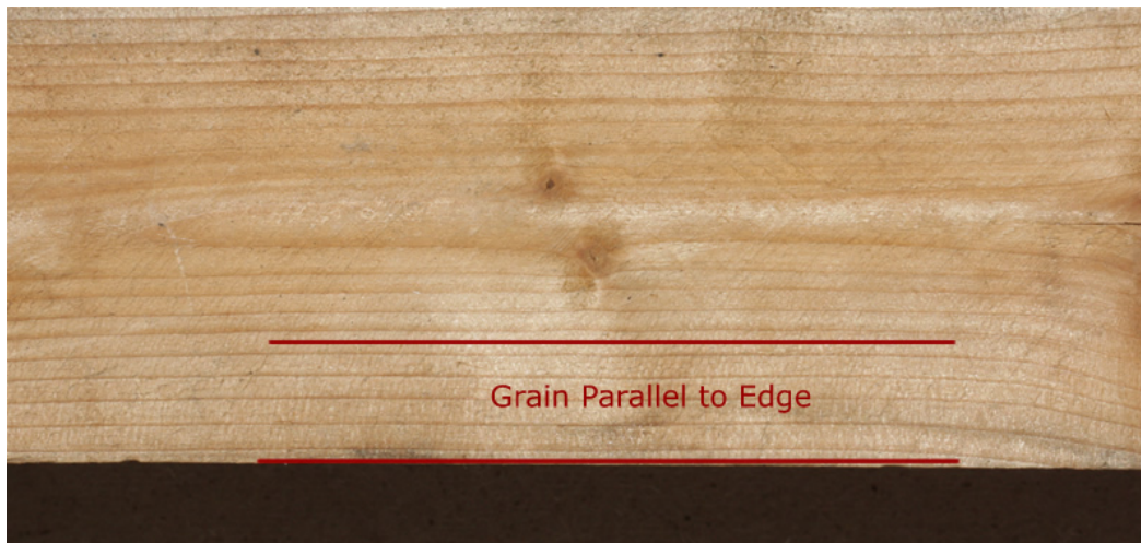
Figure 2: [SOP_SHO 004] Grain Parallel to Timber length
